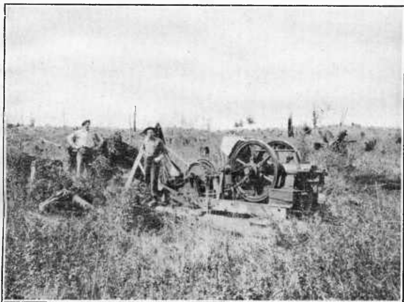
FIG. 10.—A small gasoline donkey engine used in pulling stumps.
